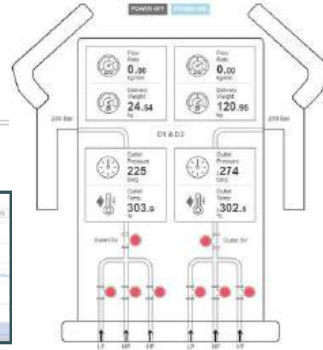
An insight into the complexity of SCADA, showing a live overview of a dispenser
